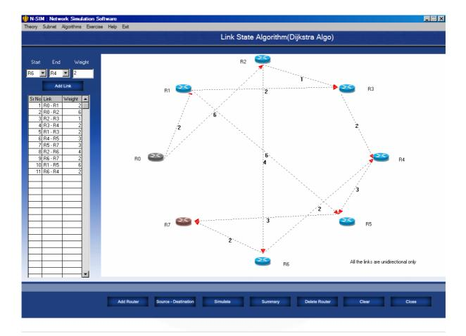
10. To simulate and find out shortest path select the source and destination routers.
