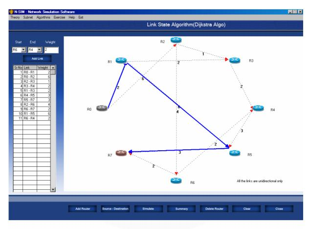
11. Click on simulate button to start the algorithm, this will calculate the shortest path and will be shown on the screen.
